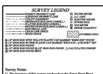
1). The bearings of this survey are based on the Texas State Plane Coordinate System, Central Zone, NAD83(2011) EPOCH 2010, and boundary referenced to 1/2", 3/8" and 5/8" iron rods found and referred to the previous recorded plat.
